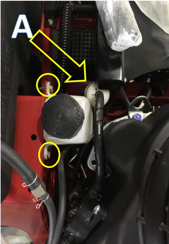
**A** Original fuel filter Location. Remove two fasteners holding expansion tank using a 10mm wrench.
