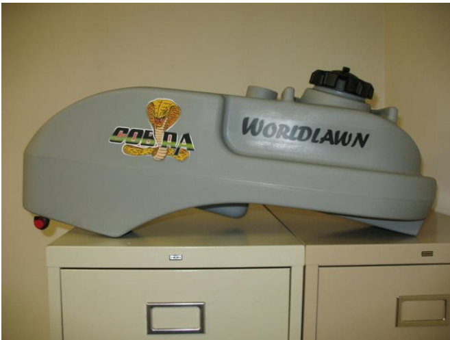
“NEW-STYLE” TANK WITH VALVE ON BOTTOM OF TANK-Replaces 2008 THRU 2009 models. Attempt to replace all units with their original valve design.
