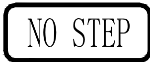
Location 1: On Top of Mower Deck Belt Shields, Left and Right Sides
