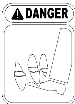
1. Cutting/dismemberment of foot by auger
